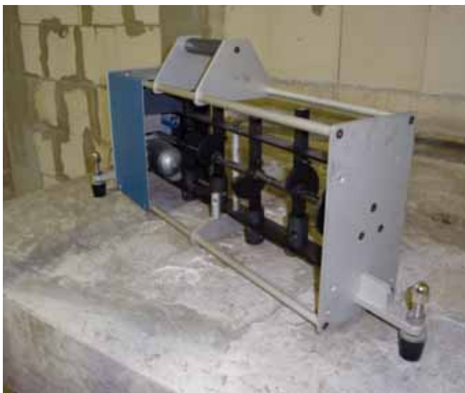
Standardised tapping machine according to EN ISO 10140
